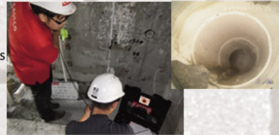
Microwave Tomography for Water Seepage Investigation
